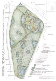
Above: A reedbed-biomass-lake system for sewage treatment, costing less than 10% of conventional sewerage costs and producing a major (biomass) energy byproduct. Such systems have now been constructed in other countries very successfully, treating over 8 million gallons of waste per day at single sites. In the UK they are not presently permitted by the water industry regulators! They are an ideal approach for community based groups like RBAG.
